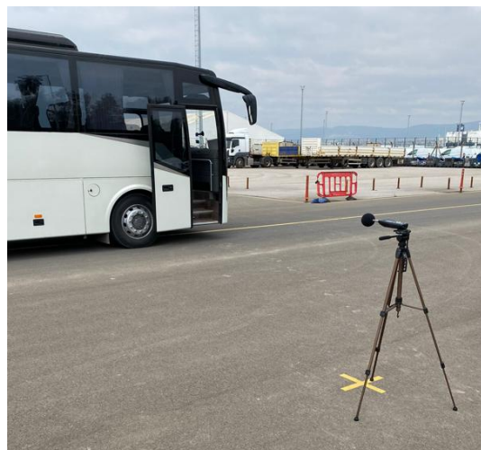
Figure 1: ECE R51 pass-by noise test setup showing the microphone position at the test track during vehicle noise measurements.
